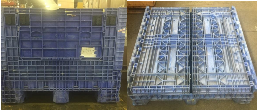
Containers should be stackable and/or collapsible
